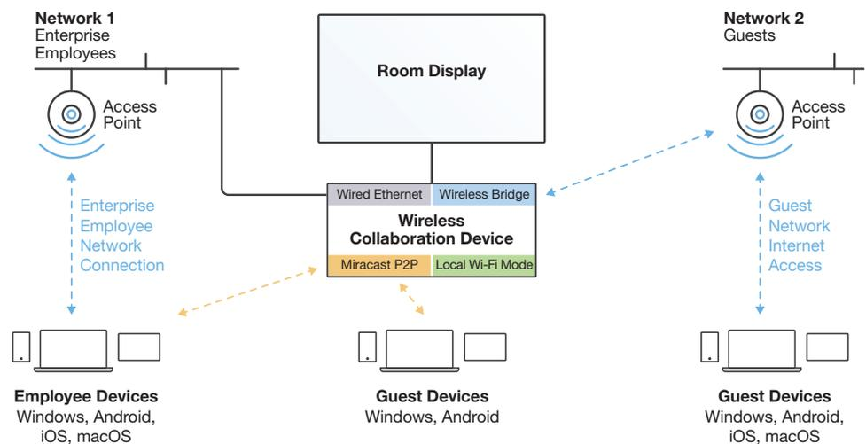
Essentially, all constraints for security, network, management and user deployment are met. No apps or USB dongles are used, no added training is required, and users of all major operating systems can be accommodated. Simultaneous network access is enabled for employees and guests. Management of the device's bands, channels and power for Miracast P2P ensures optimal user experience and co-existence with existing nearby enterprise Wi-Fi access points. Touch screens are supported when available.
