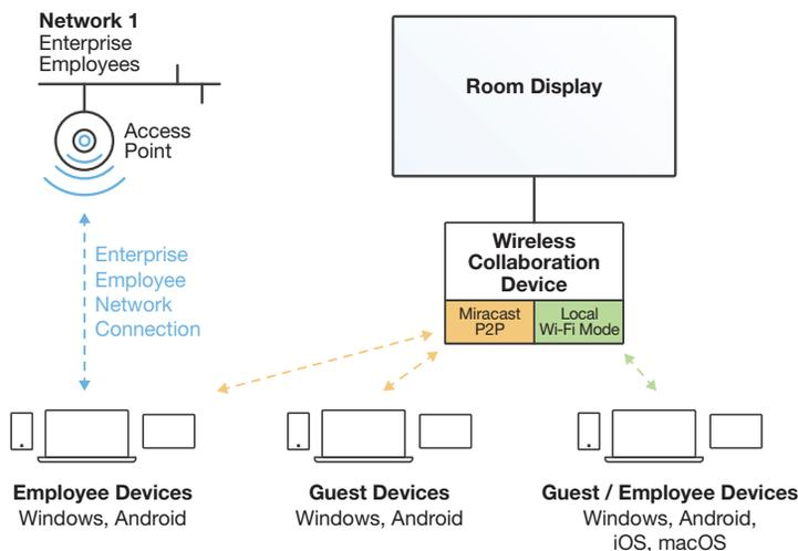
All constraints for security, network, management and user deployment are met. No apps or USB dongles are used, no added training is required, and users of all major operating systems can be accommodated. Management of the device's bands, channels and power for Miracast P2P and local Wi-Fi access point ensures optimal user experience and co-existence with existing nearby Wi-Fi access points. Touch screens are supported when available.
