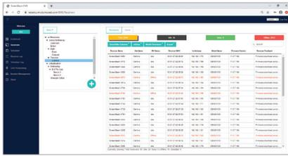
Every 1100 Plus receiver includes Central Management Enterprise software to monitor and manage ScreenBeam receivers using a standard web browser, and support multi-user and role-based access for large deployments with multiple sites and administrators. [Learn More](#)
