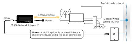
**IMPORTANT:** An existing MoCA-ready network or another ECB7250 Adapter is required. Internet availability should be delivered from your Internet service provider device (i.e., Cable or Fios modem/router).
