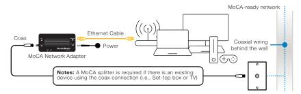
**IMPORTANT:** An existing MoCA-ready network or another ECB6200 Adapter is required. Internet availability should be delivered from your Internet service provider device (i.e., Cable or Fios modem/router).
