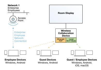
All constraints for security, network, management and user deployment are met. No apps or USB dongles are used, no added training is required, and users of all major operating systems can be accommodated. Management of the device's bands, channels and power for Miracast P2P AGO and local Wi-Fi access point ensures optimal user experience and co-existence with existing nearby Wi-Fi access points. Touch screens are supported when available.
